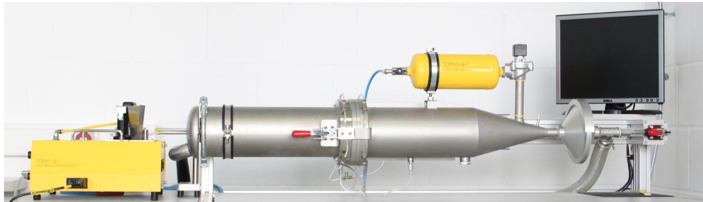
Figure 1: Test rig according to VDI3926
